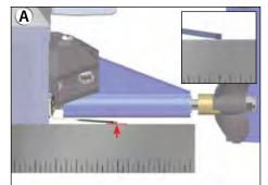
Hold a straightedge against the hull so it extends past the trim tab. The tab will rest on the straightedge or be within 1mm of its edge. This is the stock setting. Rigorous testing has shown this setting to offer the best handling in most conditions.
