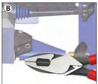
To adjust the trim tab, grip it securely with a pair of pliers as close to the bend as possible. Flex the trim tab down to set a new angle. Note that the trim tab has some spring-back, and will need to be flexed slightly farther than the actual position you wish to set.
