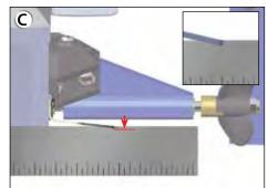
This illustration shows 1mm of downward defection. This small setting will cause a significant change in the hull's attitude. Settings of 2-3mm deflection should be considered the maximum.
