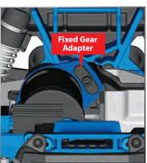
If you choose to do so, you can also set the gear mesh manually without using the fixed gear adapter. With the adapter removed, loosen the motor screw. Cut a narrow strip of notebook paper and run it into the gear mesh. Slide the motor and pinion gear into the spur gear. Retighten the motor
