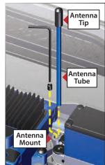
When reinstalling the antenna, first slide the antenna wire into the bottom of the antenna tube until the white
